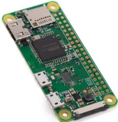
The Raspberry Pi Zero W extends the Pi Zero family and comes with added wireless LAN and Bluetooth connectivity.
